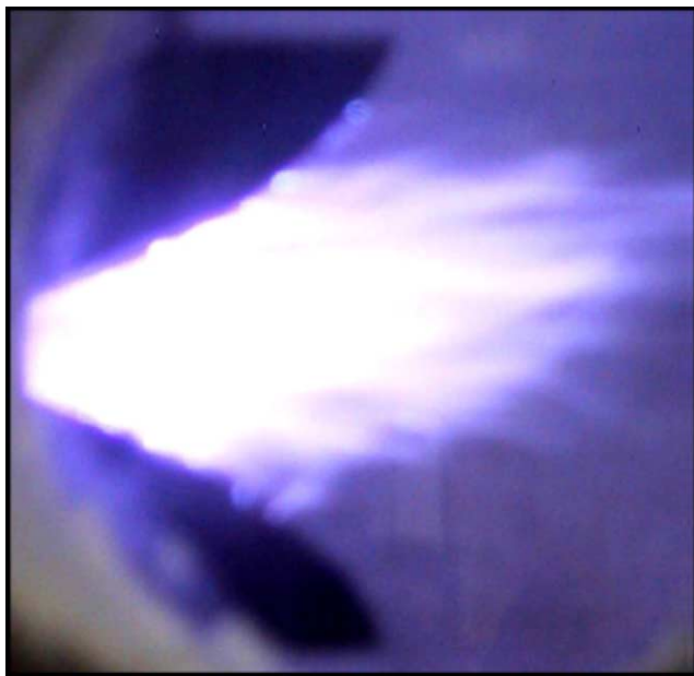
Fig. 4. The gliding discharge in hot air and water (temperature: 573 K, pressure: 2 \times 10^5 Pa).
